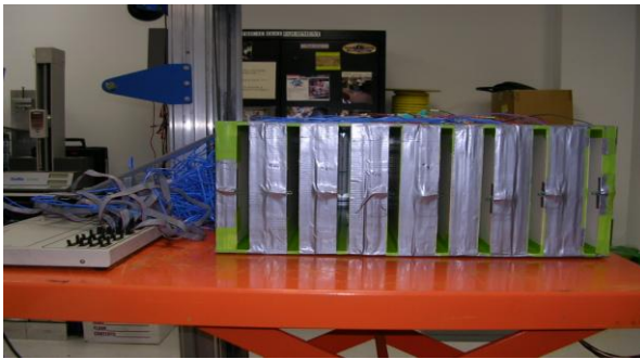
Figure 4: Calibration setup for sub-system level mockup of modules SA
