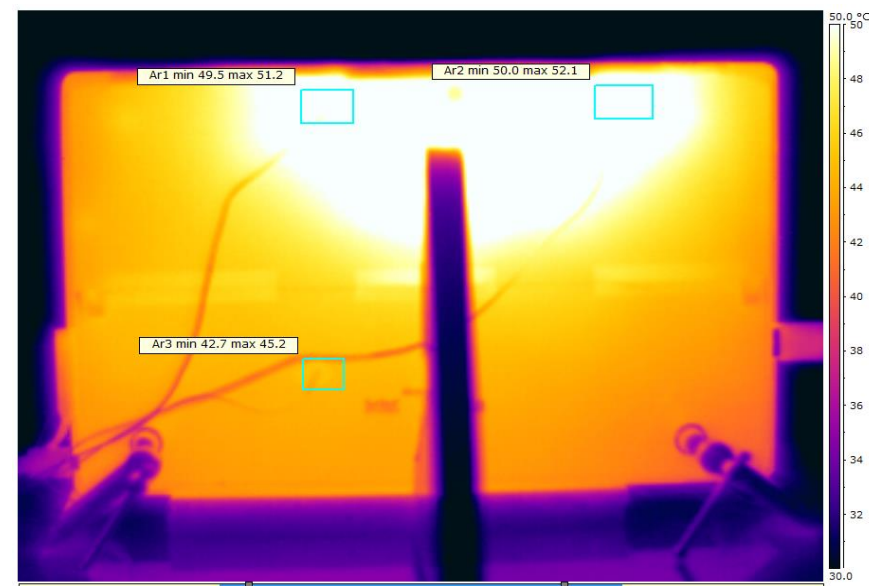
Enhanced Spreading (case 2) with Blower @ 3900 RPM
