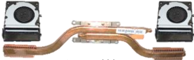
Heatpipes and blowers
